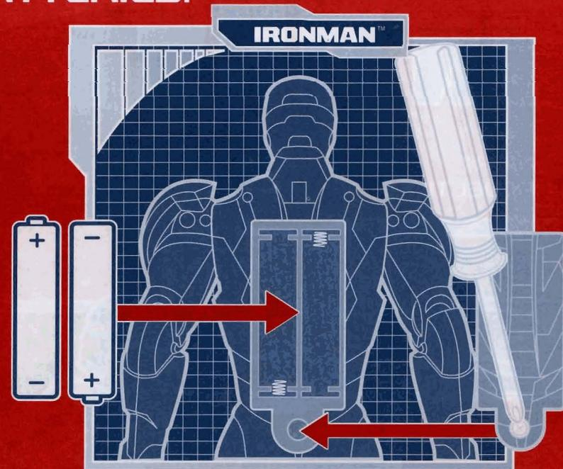
Use a Phillips/cross head screwdriver (not included) to loosen screw in battery compartment door (screw remains attached to door). Remove door and discard old batteries. Insert 2 x 1.5V fresh "AAA" or R03 size batteries. Alkaline batteries recommended. Replace door and tighten screw.
