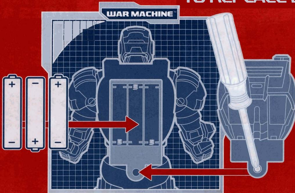
Use a Phillips/cross head screwdriver (not included) to loosen screw in battery compartment door (screw remains attached to door). Remove door and discard old batteries. Insert 3 x 1.5V fresh "AAA" or R03 size batteries. Alkaline batteries recommended. Replace door and tighten screw.
